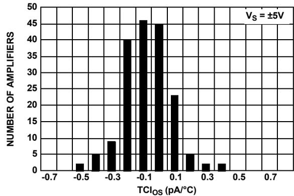
FIGURE 20. TC<sub>1os-</sub>-vs NUMBER OF AMPLIFIERS, V<sub>S</sub> = ±5V
