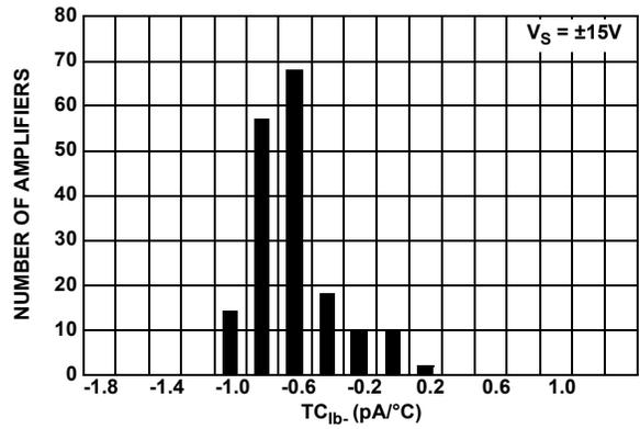
FIGURE 16. TC<sub>1b</sub>-vs NUMBER OF AMPLIFIERS, V<sub>S</sub> = ±15V
