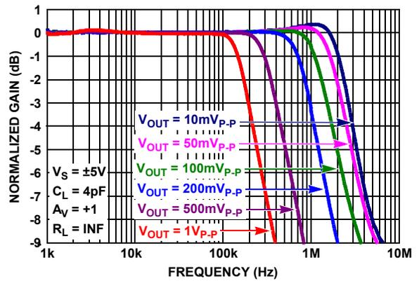
FIGURE 46. GAIN vs FREQUENCY vs OUTPUT VOLTAGE
