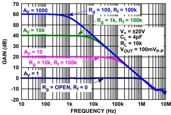
FIGURE 60. CHARACTERIZED CLOSED LOOP GAIN vs FREQUENCY
