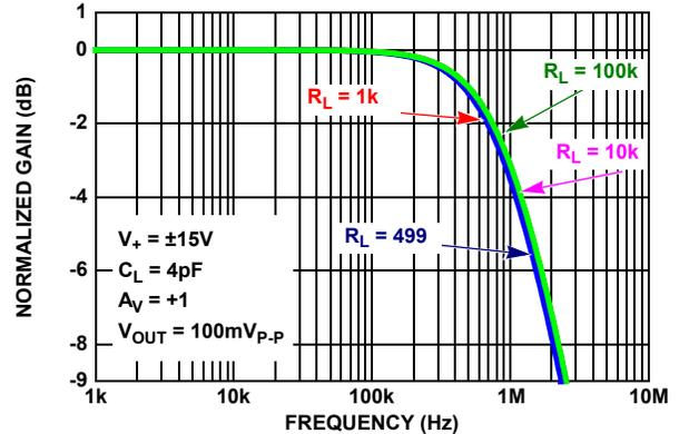
FIGURE 63. SIMULATED CLOSED LOOP GAIN vs  $R_L$
