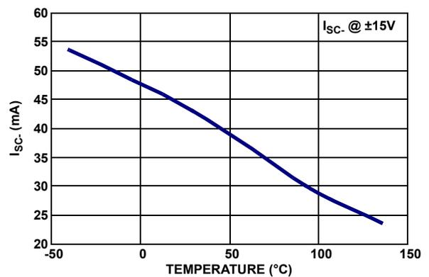
FIGURE 32. NEGATIVE SHORT CIRCUIT CURRENT vs TEMPERATURE
