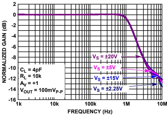
FIGURE 47. GAIN vs FREQUENCY vs SUPPLY VOLTAGE
