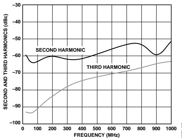
Figure 9. Single-Tone Harmonics vs. Frequency,  $P_{out} = 0 \text{ dBm}$
