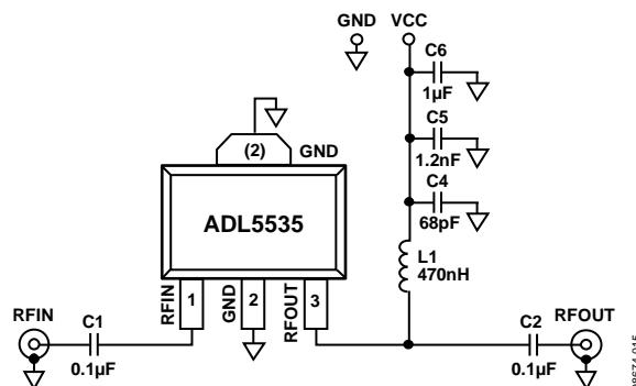
Figure 16. Basic Connections
