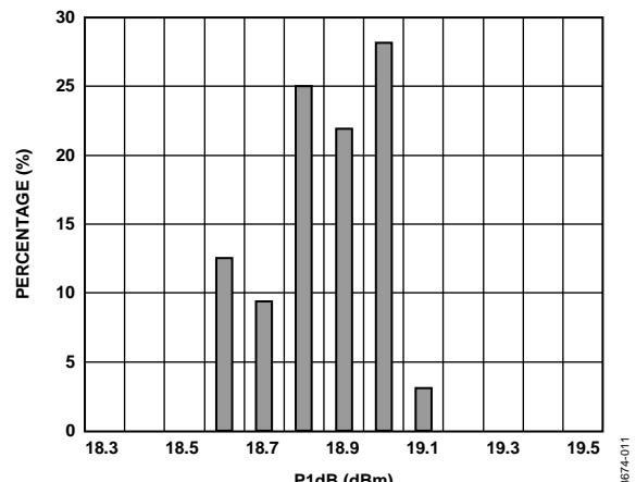
Figure 11. P1dB Distribution at 190 MHz
