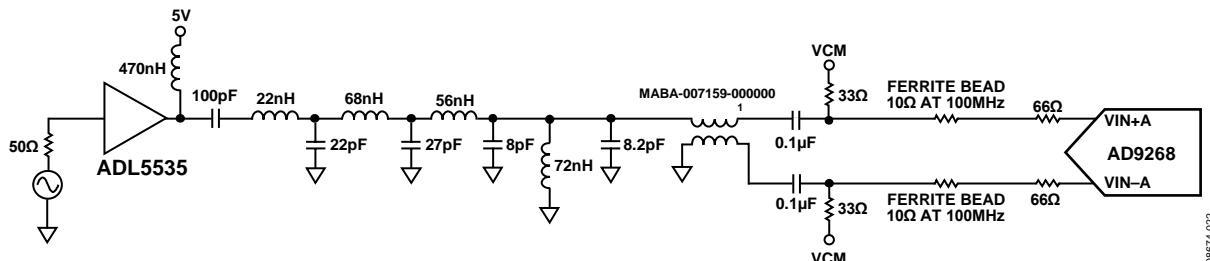
Figure 23. Schematic of the **ADL5535** Driving the **AD9268** 16-Bit ADC
