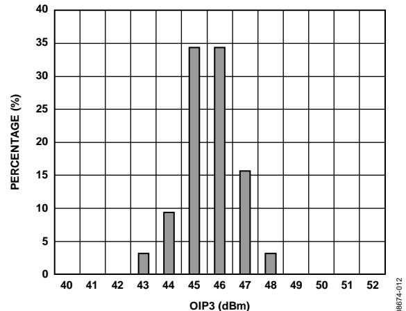
Figure 12. OIP3 Distribution at 190 MHz,  $P_{out} = 3 \text{ dBm}$
