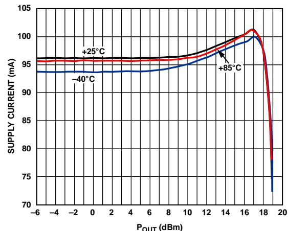
Figure 15. Supply Current vs.  $P_{OUT}$  at Various Temperatures
