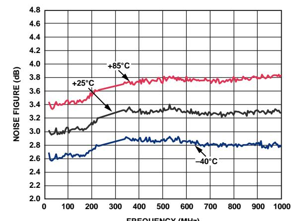
Figure 8. Noise Figure vs. Frequency and Temperature
