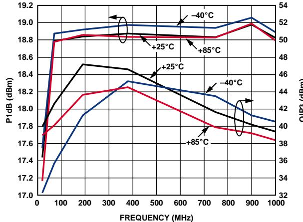
Figure 6. P1dB and OIP3 vs. Frequency and Temperature
