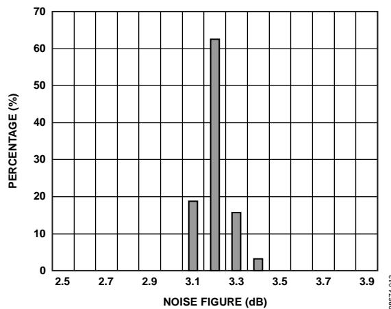
Figure 13. Noise Figure Distribution at 190 MHz
