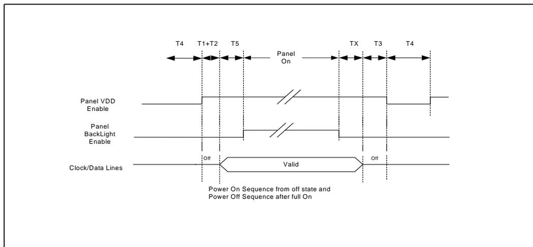
**Note:** Support for programming parameters TX and T1 through T5 using software is provided.
