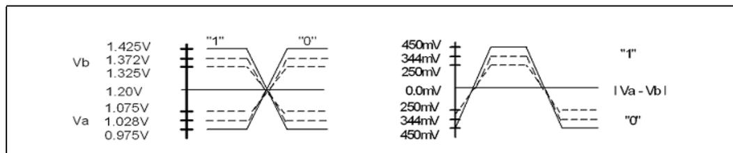
1s and 0s are represented the differential voltage between the pair of signals. As shown in the figure below a serial pattern of 110011 represents one cycle of the clock.
