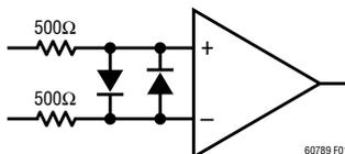
Figure 1. Op Amp with Input Voltage Clamp
