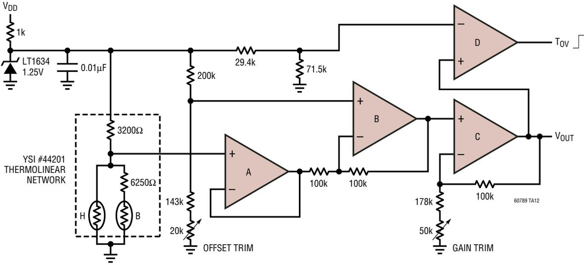
A TO D: LTC6079,  $V_{DD} = 2.7V$  TO  $5.5V$ ,  $V_{SS} = GND$
