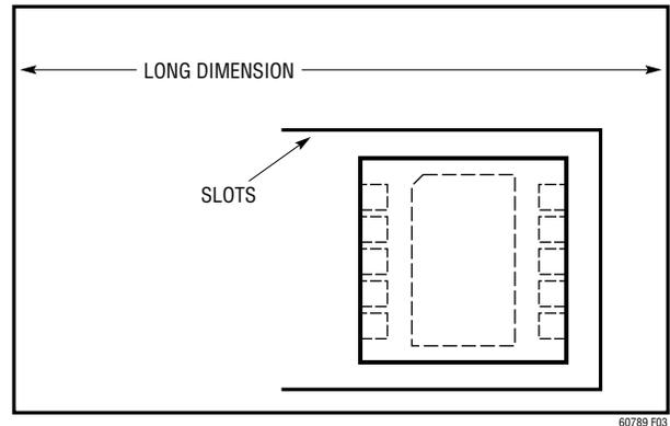
Figure 3. Vertical Orientation of LTC6078DD with Slots
