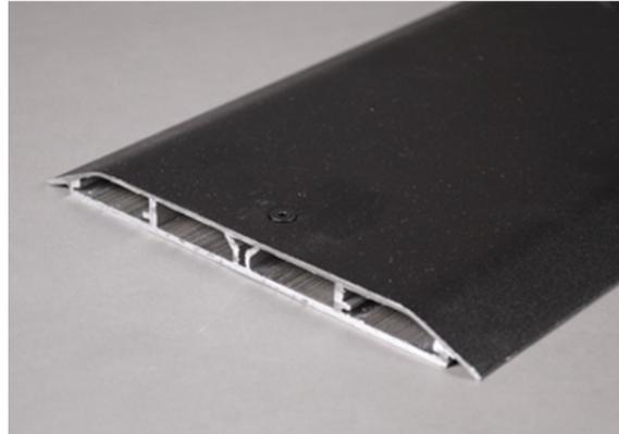
Cover: 0.040" (1.0mm) steel. Base: 0.080" (2.0mm) aluminum. Durable black powder coat finish. Divided into four channels. Packed one (1) 8' (2.4m) length of base and cover per carton. NOTE: Not recommended for use in high traffic areas.
