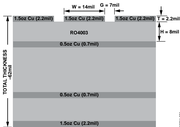
Figure 22. Probe Matrix Board (Cross Section View)
