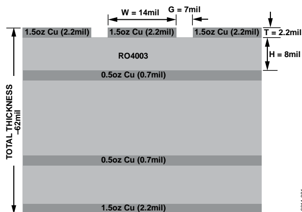
Figure 22. Probe Matrix Board (Cross Section View)
