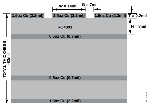
Figure 22. Probe Matrix Board (Cross Section View)
