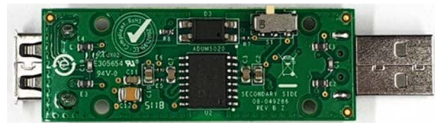
Figure 4. S1 Switch Position for Low Speed Operation
