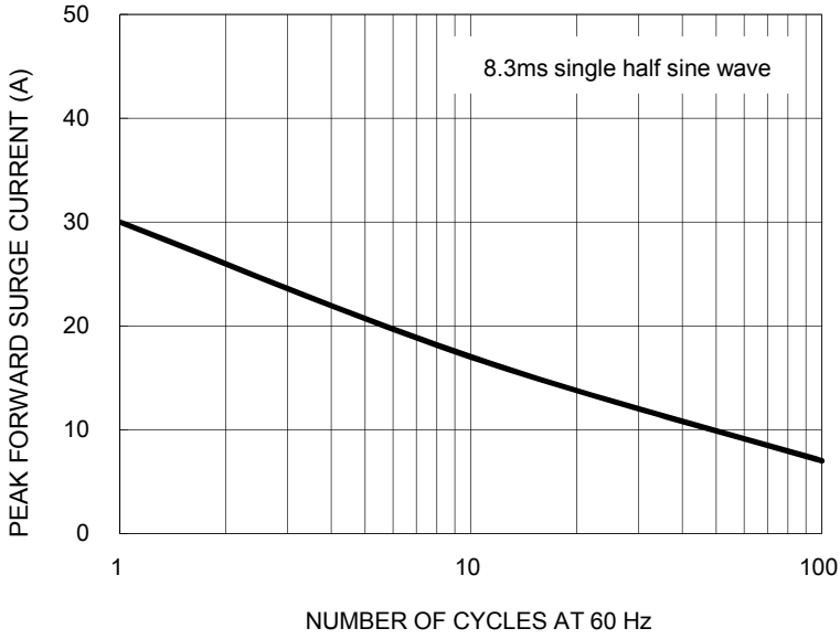
FIG. 3 MAXIMUM NON-REPETITIVE FORWARD SURGE CURRENT
