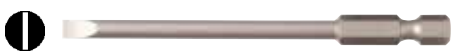
760 Slotted Power Blades S2 modified tool steel. Hardened & tempered to HRC 60. Blades fit CentroFix power blade handle. OAL 90mm/3.5".
