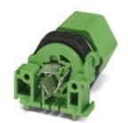
Panel feed-through, for internal wall mounting, with dip-solder connection, length of the solder pin: 3.8 mm, hole  $\emptyset$  3-pos. = 20.8 mm - 0.3 mm
