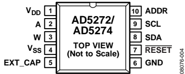
Figure 4. MSOP Pin Configuration
