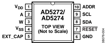
Figure 4. MSOP Pin Configuration
