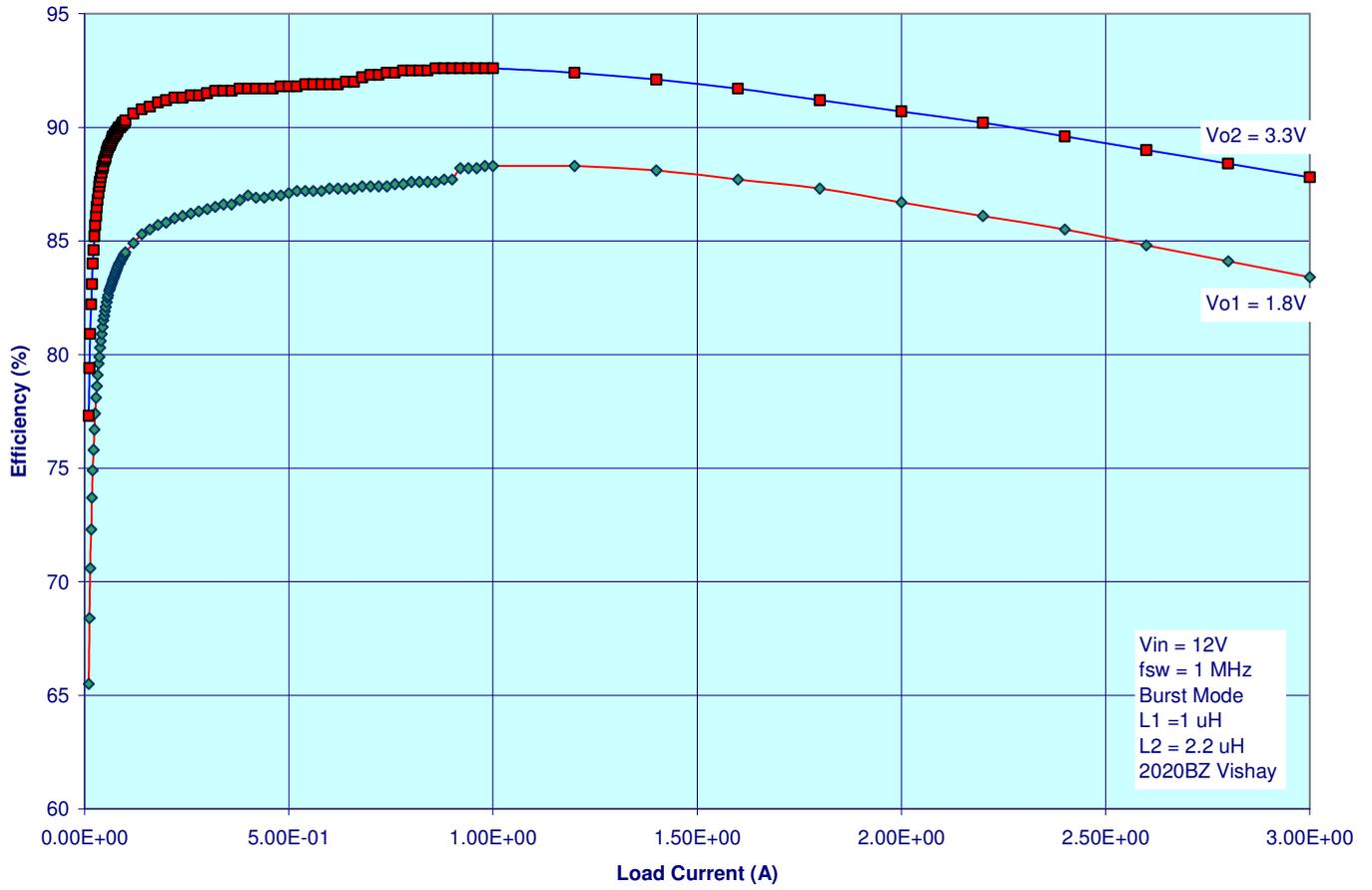
Figure 5. LTC3633 DC1347 Efficiency
