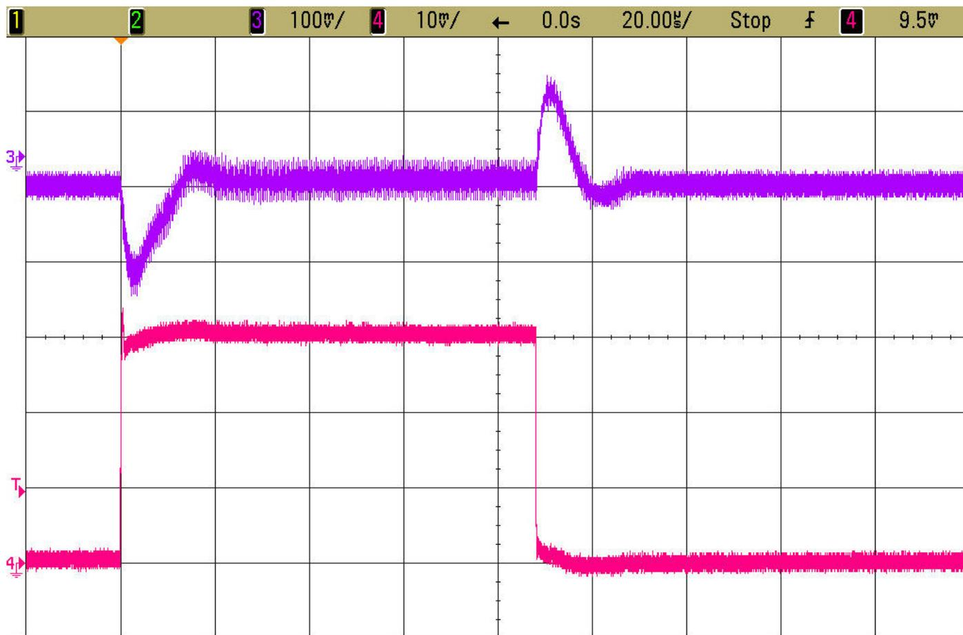
Figure 4.  $V_{OUT2}$  Load Step Response
