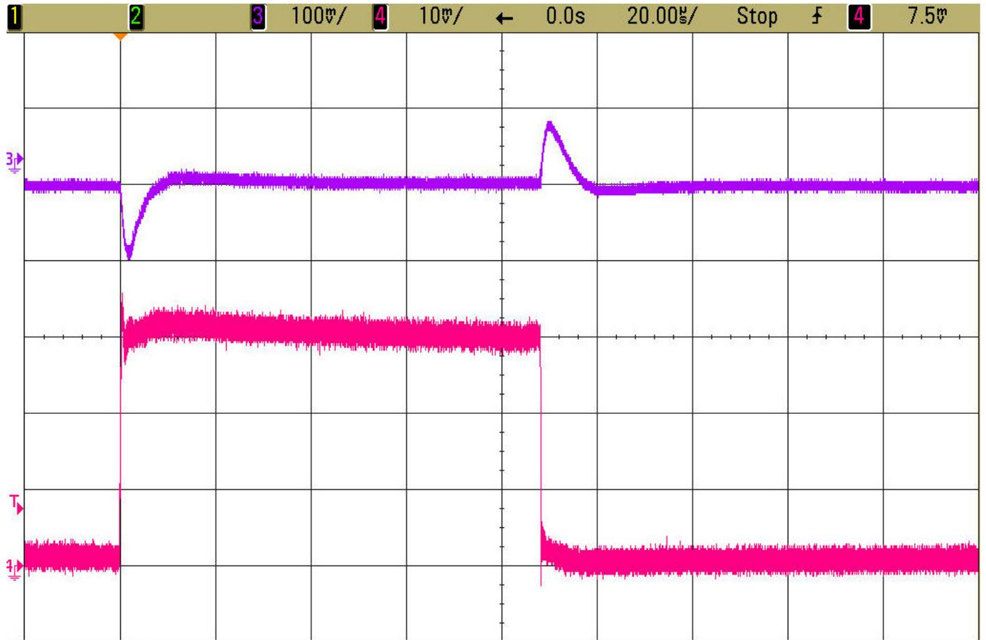
Figure 3.  $V_{OUT1}$  Load Step Response
