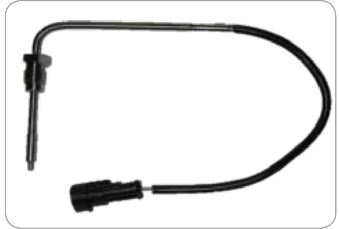
This sensor operates over a temperature range from  $-40^{\circ}\text{C}$  to  $850^{\circ}\text{C}$ . It monitors the temperature before and after SCR system in the diesel engines as part of the engine control strategy. It is designed for fast response, optimized for thermal dissipation and suitable for high vibration and corrosive environments.
