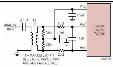
Figure 2. Analog Front End Circuit For 1MHz < A<sub>IN</sub> < 70MHz (1 of 2)
