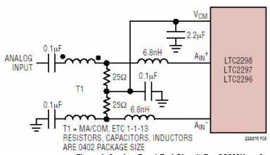
Figure 4. Analog Front End Circuit For 300MHz <  $A_{\mbox{\footnotesize{IN}}}$  < 500MHz
