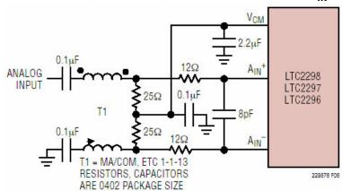
Figure 3. Analog Front End Circuit For 70MHz  $< A_{IN} < 170MHz$  (1 of 2)
