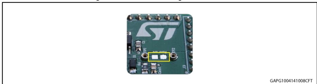
Figure 5: Pads for soldering SMD resistor
