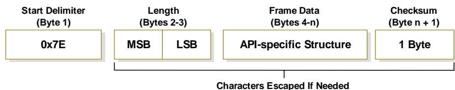
Figure 6-07. UART Data Frame Structure - with escape control characters:
