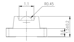
For reflow soldering (propose)
