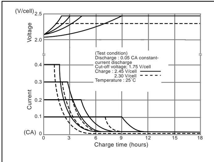
In order to fully utilize the characteristics of VRLA batteries, constant-voltage charging is recommended. For details of charging see page 19.
