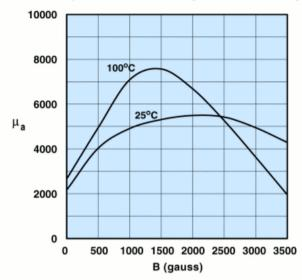
Measured on an 18/10/6mm toroid at 10kHz.
