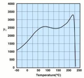
Measured on an 18/10/6mm toroid at 100kHz.
