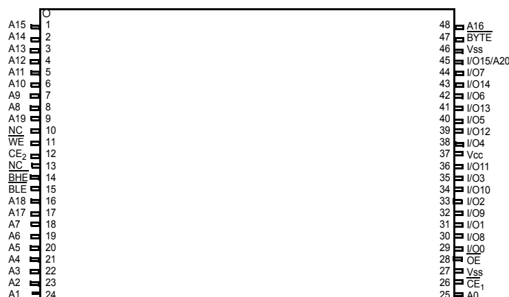
Figure 2. 48-pin TSOP I pinout (Top View) [2, 3]
