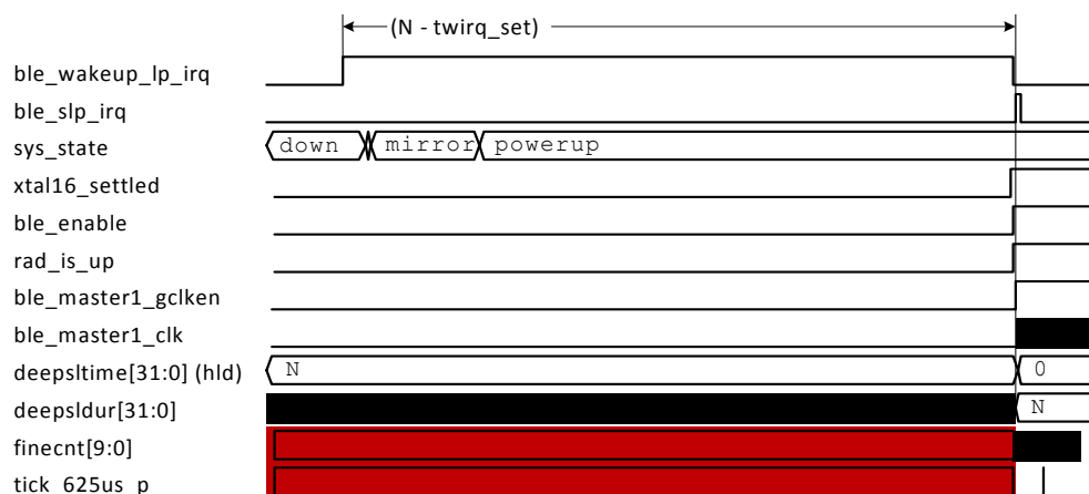
Figure 118: Exit BLE Deep Sleep Mode at predetermined time (zoom out)
