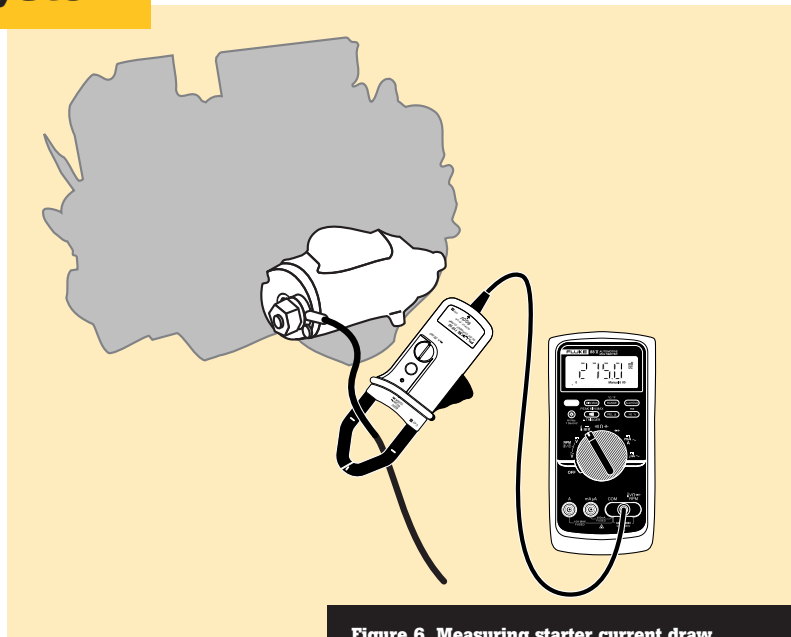
Figure 6. Measuring starter current draw
