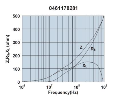
Impedance, reactance, and resistance vs. frequency.
