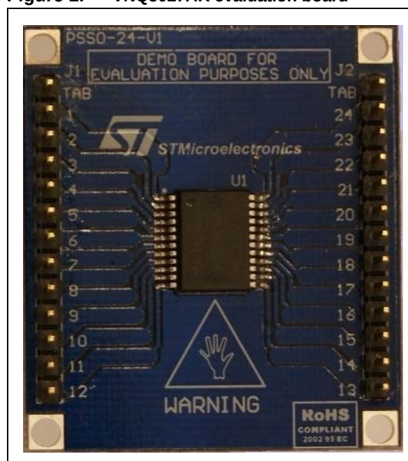
Figure 1. VNQ5027AK evaluation board
