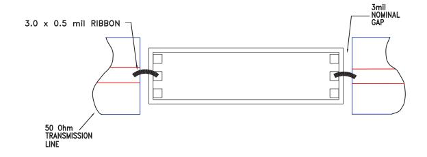
Note 1: Best performance obtained from use of <10 mil (long) by 3 by 0.5 mil ribbons on input and output.
