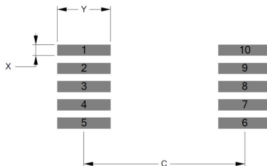
**Figure 12.2 MSOP-10 Footprint.**
