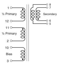
Primary windings to be connected in series and secondary windings to be connected in parallel on the PC board.
