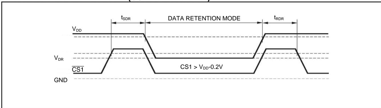
**DATA RETENTION WAVEFORM (CS2 CONTROLLED)**
