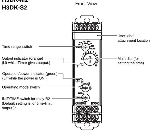
\*If the switch is left between settings, proper operation may not be possible. Make sure that the switch is set properly.
