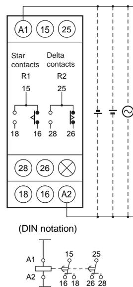
Note: The power supply terminals do not have polarity.
