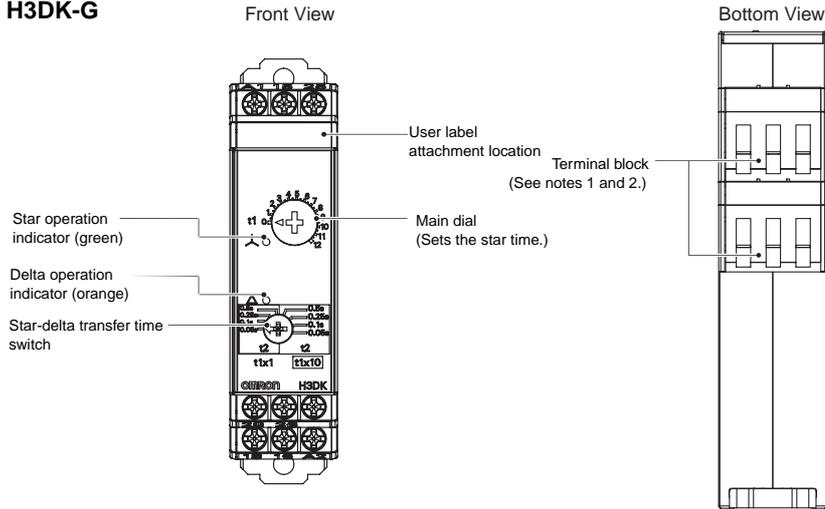
Note 1. Use solid wire (2.5 mm<sup>2</sup> max.) or ferrules with insulative sleeves to connect to the terminals.
