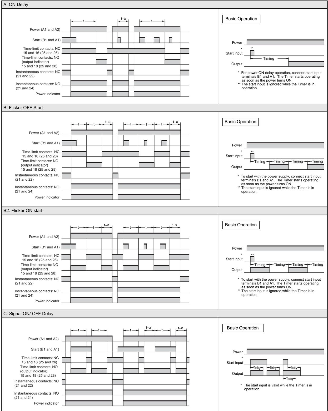
Note 1. The reset time is 0.1 s min. Make sure the signal input time is 0.05 s or longer.
