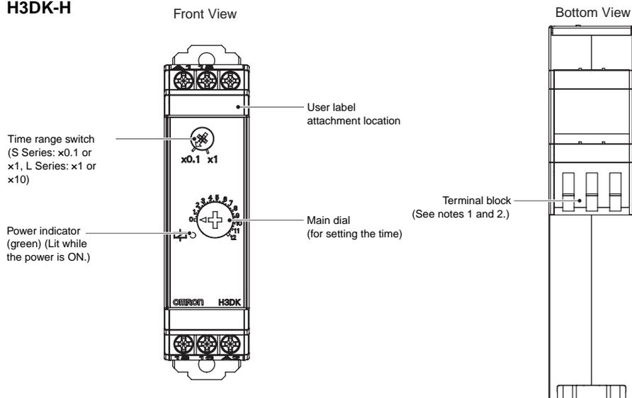
Note 1. Use solid wire (2.5 mm<sup>2</sup> max.) or ferrules with insulative sleeves to connect to the terminals. To maintain the withstand voltage after connecting the terminals, insert no more than 8 mm of exposed conductor into the terminal.
