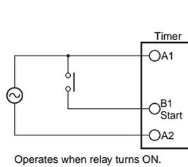
Consider the minimum load of the relay. (See signal levels on the right.)
