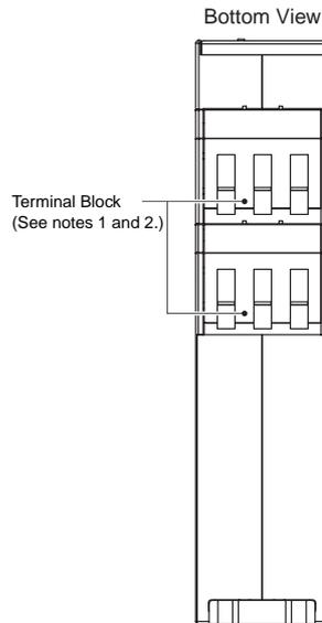
Note 1. Use solid wire (2.5 mm<sup>2</sup> max.) or ferrules with insulative sleeves to connect to the terminals.
