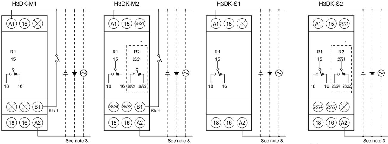
Note 1: The time-limit contact symbol for previous models of Timers was . The time-limit contact symbol for the H3DK is . A different symbol is used because the H3DK supports multiple operating modes.
