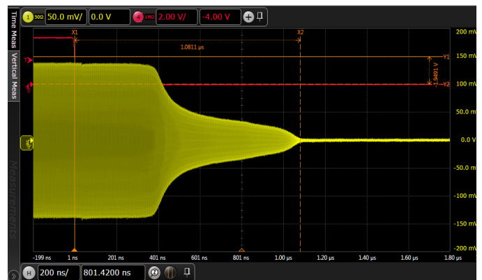
Figure 25. Switching Time [Insertion Loss to Isolation State]
