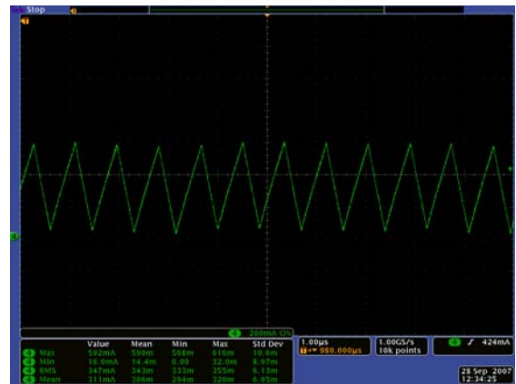
FIGURE 12. I L ZOOM IN AT PWM DIMMING ZOOM IN
