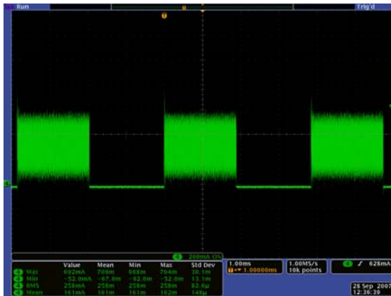
FIGURE 11. IL AT 50% PWM DIMMING
