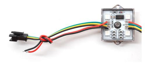
Wiring is pretty easy since there are only 4 wires. The only important thing is that you should not try to power the LED
