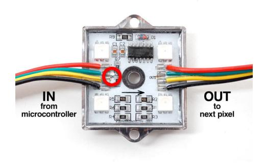
The pixel strands include plugs for joining multiple strands, plus two wires for connecting power:
