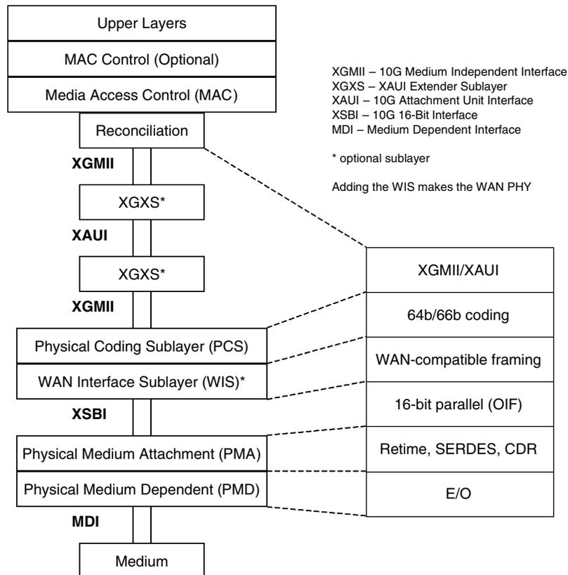
Figure 2-2. XAUI Solution Simplified Block Diagram
