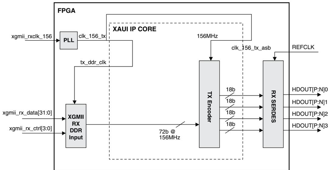
Figure 2-7. XAUI IP Core Transmit Direction Data Translations
