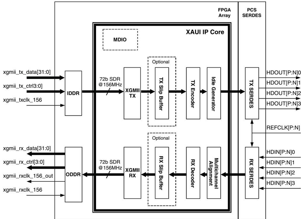
Figure 2-3. XAUI IP Core I/O
