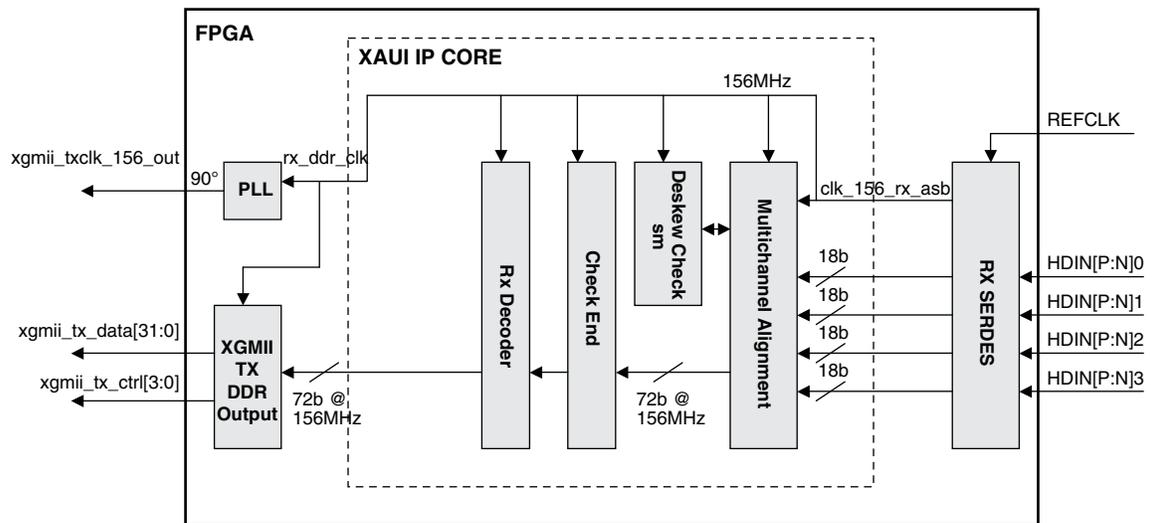
Figure 2-5. XAUI IP Core Receive Direction Data Translations
