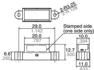
\*Rear side connector protrusion: Max. 0.4mm
