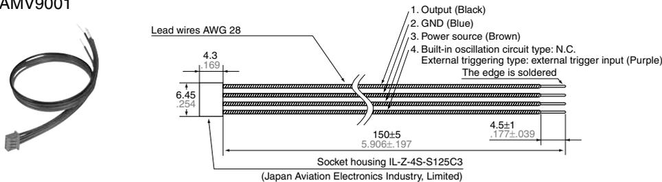
Note: Mistaken cable assembly can cause damage to the internal circuits, so please check the power cord before switching ON. (Particular care must be taken as to avoid reverse connection of the power.)
