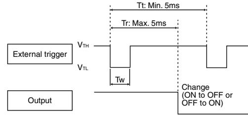
Note: The sensor recognizes at the  $V_{TH} \rightarrow V_{TL}$  edge of an external trigger that the external trigger has been input.
