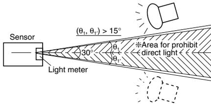
Note: Light from direct light sources (sunlight, strobe light, inverter illumination, reflected light from glass or mirrors etc.) that enters the sensor from within the prohibited range can cause the sensor to operate erroneously.
