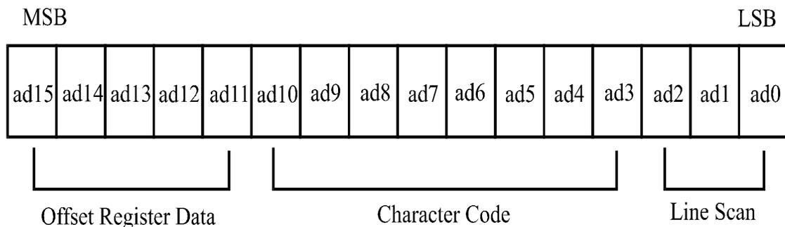
T6963C assign External character generator, when character code set 80H TO FFH in using internal character generator. Character code 00H to 80H assign External character generator, when
