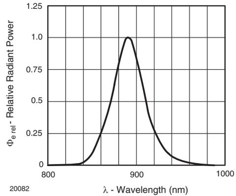
Fig. 6 - Relative Radiant Power vs. Wavelength
