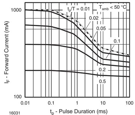
Fig. 8 - Pulse Forward Current vs. Pulse Duration
