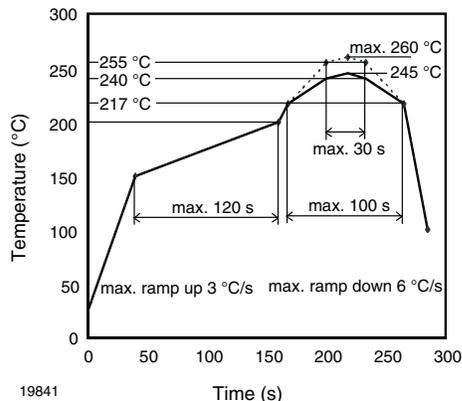
Fig. 9 - Lead (Pb)-free Reflow Solder Profile acc. J-STD-020
