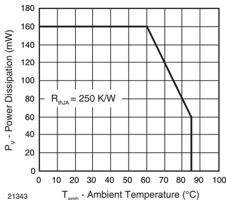
Fig. 1 - Power Dissipation Limit vs. Ambient Temperature
