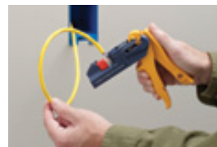
3. Insert jack in JackRapid front first with IDC slots facing blades of JackRapid.
