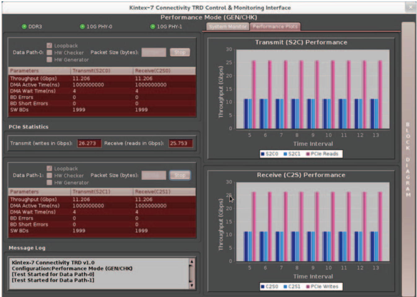
Figure 2-21: GEN/CHK Performance Mode Plots
