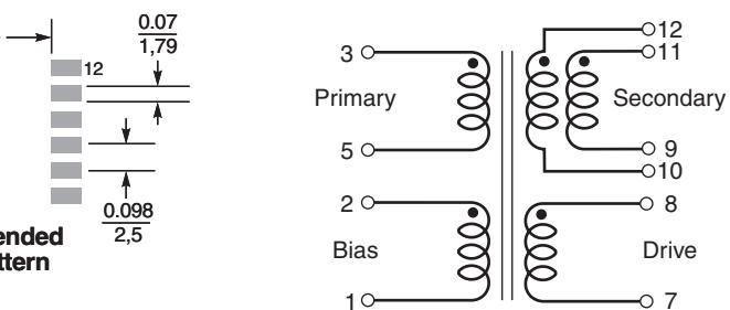
The secondary windings are to be connected in parallel on the PC board.
