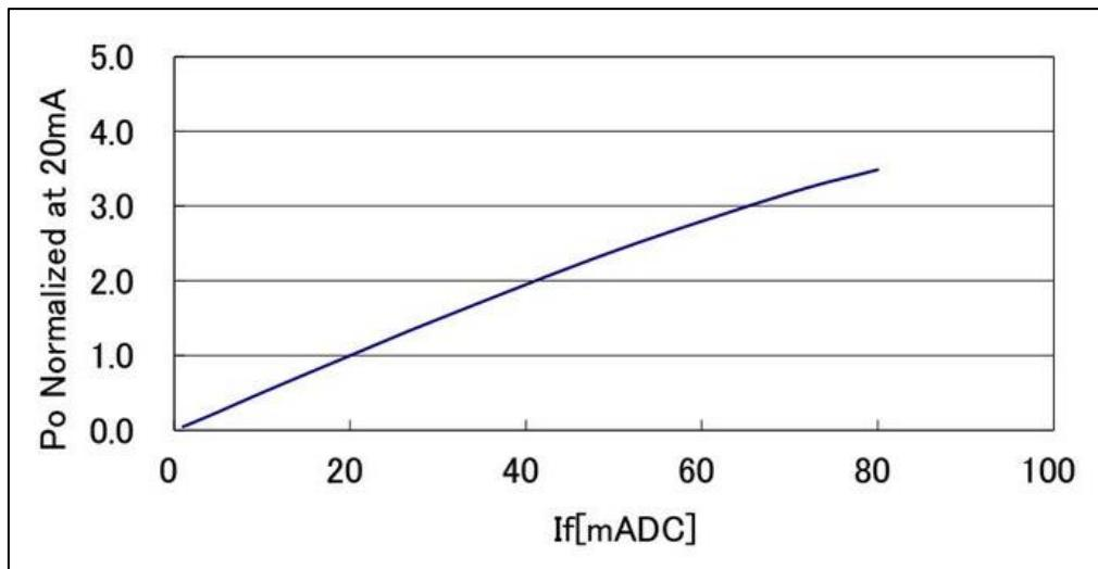
Figure 9.2 Forward LED Current vs. Normalized Radiated Power.
