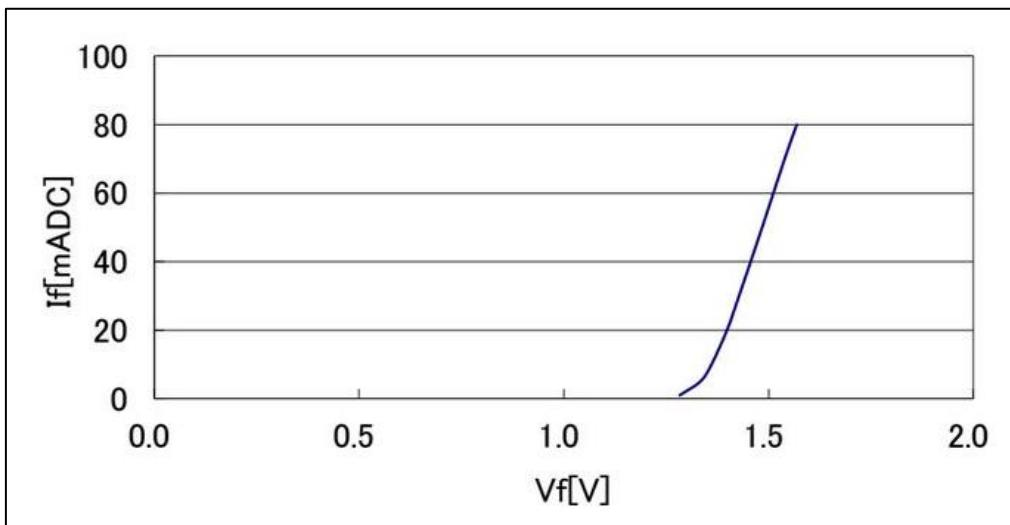
Figure 9.3 Forward LED Voltage vs. Forward LED Current.
