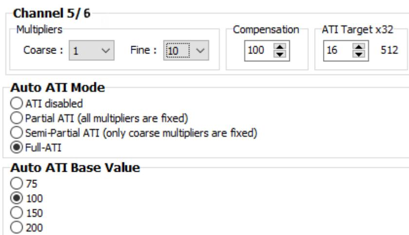
The ATI process adjusts three values (Coarse multiplier, Fine multiplier, Compensation) using two parameters per plate (ATI base and ATI target). The ATI process is used to ensure that the sensor's sensitivity is not severely affected by external influences (Temperature, voltage supply change, etc.).
