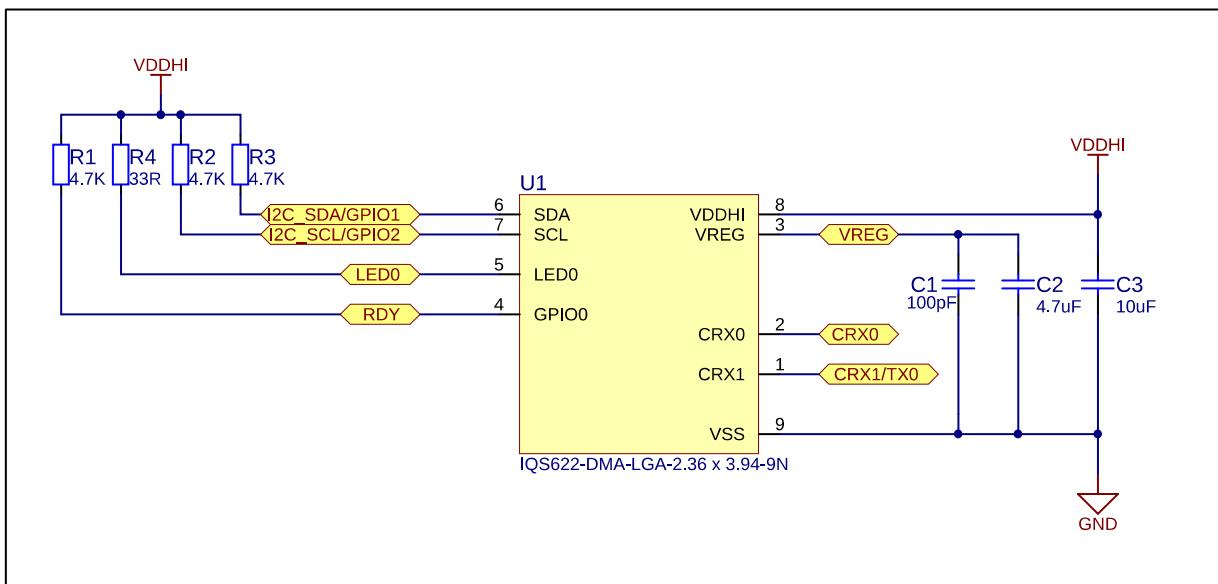
Figure 1.3 IQS622 reference schematic
