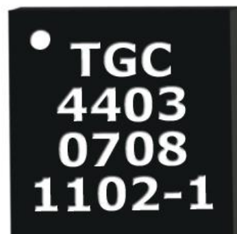
16-pin 4x4 mm QFN package
