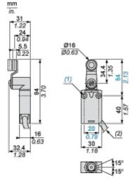
(1) 2 fixing holes  $\varnothing$  4.2 mm, counterbored  $\varnothing$  8 mm by 4 mm deep.
