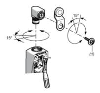
(1) Tightening torque (Min: 1) (Max: 1.5)
