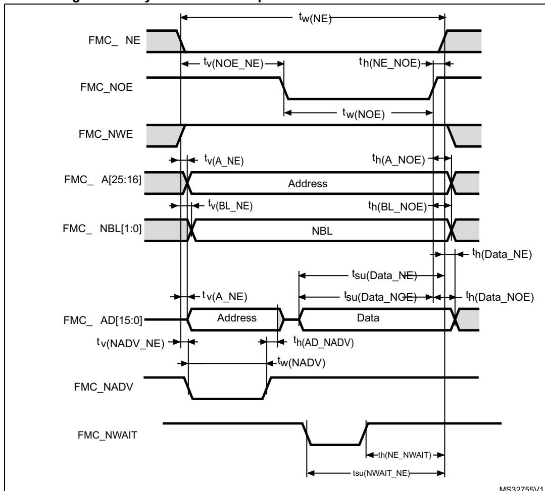
**Table 61. Asynchronous multiplexed PSRAM/NOR read timings<sup>(1)</sup>**
