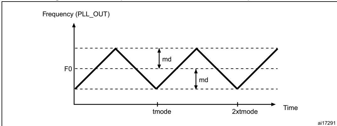
**Figure 22. PLL output clock waveforms in down spread mode**
