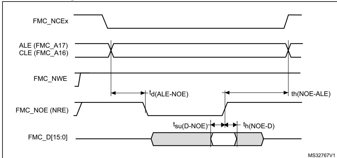
**Figure 34. NAND controller waveforms for write access**
