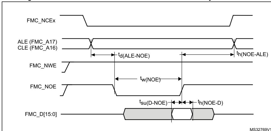
**Figure 36. NAND controller waveforms for common memory write access**
