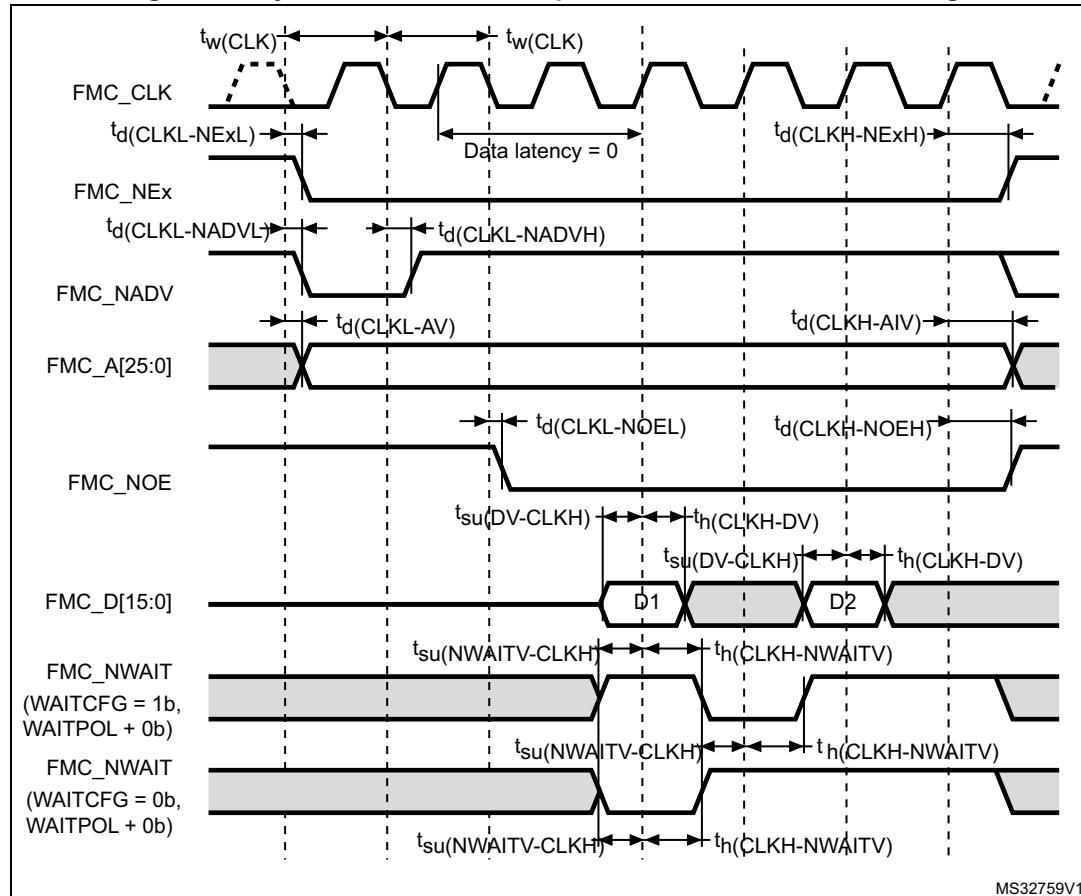
Table 67. Synchronous non-multiplexed NOR/PSRAM read timings<sup>(1)</sup>
