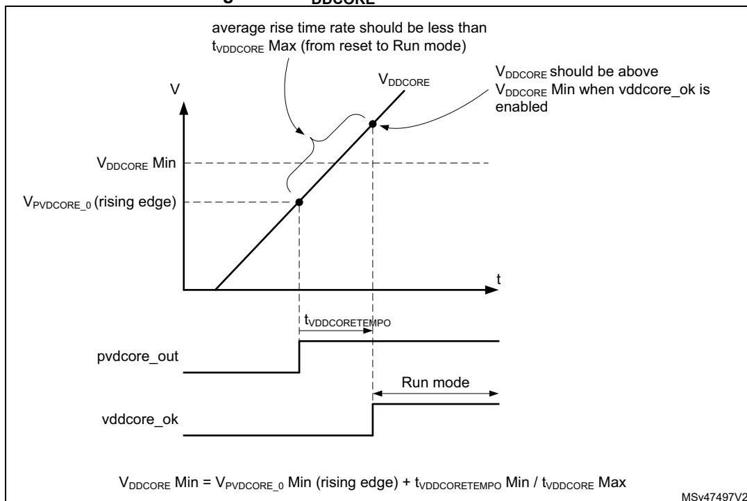
**Figure 14.  $V_{DDCORE}$  rise time from LPLV-Stop**
