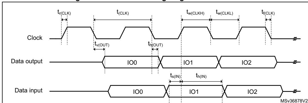
Figure 38. QUADSPI timing diagram - DDR mode
