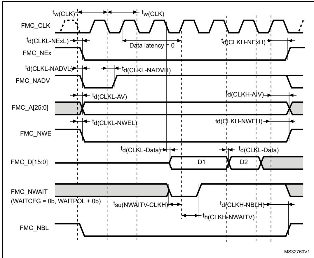
**Table 68. Synchronous non-multiplexed PSRAM write timings<sup>(1)</sup>**
