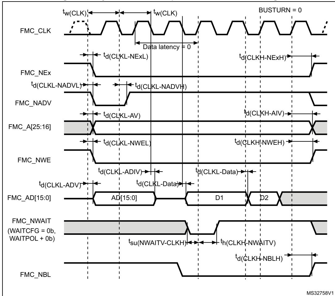
**Table 66. Synchronous multiplexed PSRAM write timings<sup>(1)</sup>**
