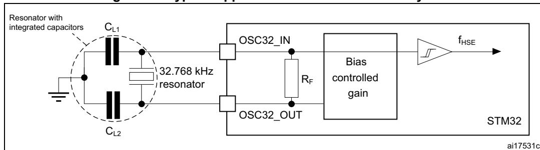
1. Adding an external resistor between OSC32\_IN and OSC32\_OUT is forbidden.
