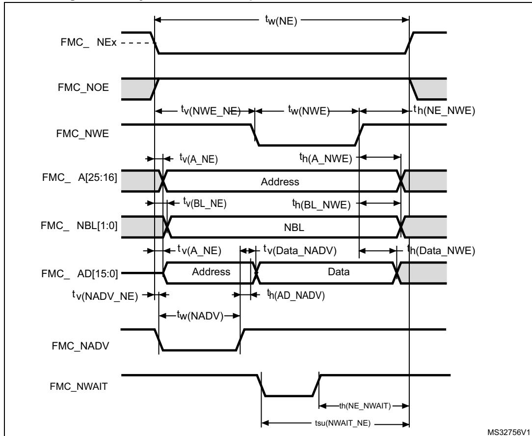
**Table 63. Asynchronous multiplexed PSRAM/NOR write timings<sup>(1)</sup>**
