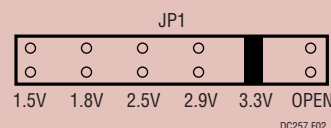
Figure 2. Output Voltage Selection (JP1) (3.3V Position Shown)
