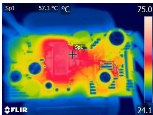
Figure 20 – Transformer Side. 265 VAC, Full Load.
