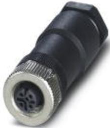
Connector, 5-position, Socket straight M12, A-coded, Screw connection, Knurl material: Zinc die-cast, nickel-plated, Cable gland Pg11, External cable diameter 8 mm ... 10 mm
